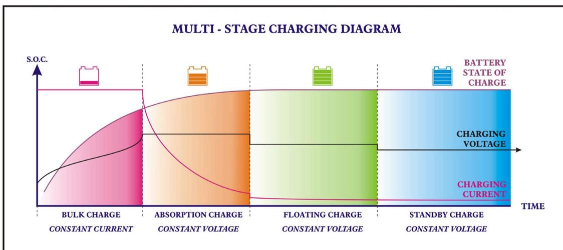
**Stage 1. THE I-PHASE. [BULK mode]** Constant current charging, Bulk LED is ON.
