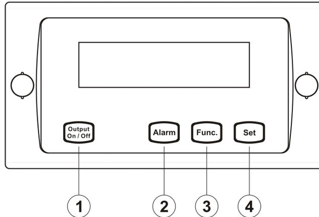
1. Output ON/OFF : To switch the charger output ON and OFF. Green LED is illuminated when output is ON.
