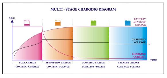
Stage 1. THE I-PHASE. [BULK mode] Constant current charging, Bulk LED is ON.
