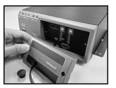
Mount back the dummy remote panel on the charger panel. d.
