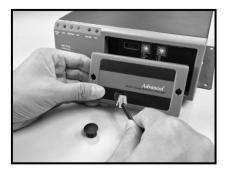
Plug in the remote cable into the charger remote socket. c.
