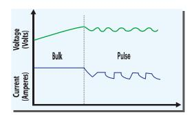
**Bulk:** This is the first stage (Constant Current) where the battery is in a low charge state. During this stage the controller delivers all of the available solar power to the Battery system.
