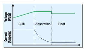
**Bulk:** This is the first stage (Constant Current) where the battery is in a low charge state. During this stage the controller delivers all of the available solar power to the Battery system.
