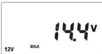
2. Press “menu” button 4 times. Window will switch to show FLOAT voltage setting. To change this setting; Press “enter” button once; you can program Float voltage via Pageup/Pagedown button:
