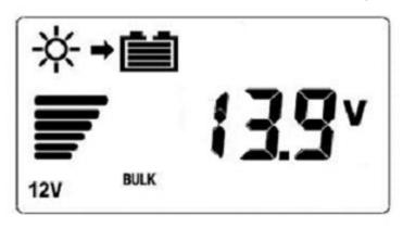
Displays Sun Icon with arrow indicating Current flow into the Battery. Displays Charging Current Bar Graph (Each bar = 5amps approx') Either Bulk or Float Mode is indicated.
