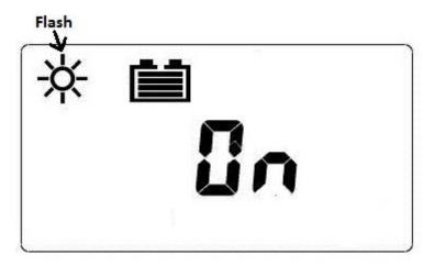
PV as Priority Source; Displays a Sun Icon Flashing & ON
