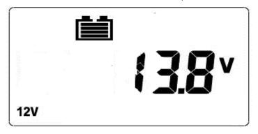
Displays just the battery voltage, with battery level.
