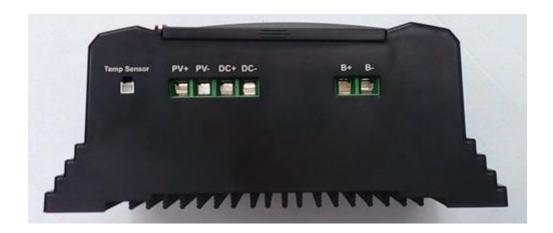
Connect PV Panel Input to; PV + and PV - Connect DC Input source to; DC + and DC - Connect your 12V battery to; B + and B -
