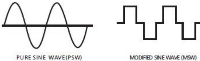
If you want to run your equipment exactly to the manufacturer's specifications, choose a *pure sine wave* inverter. With pure sine wave, motors start easier and run cooler. As well, some equipment **may only** operate properly with a pure sine wave inverter, such as laser printers, variable speed motors and digital clocks/devices.
